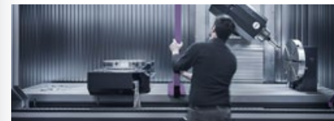
Non stop machining software and division wall of workign areas (STAR 3000).
